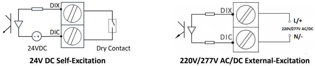
Figure 2-7 DI Connections
